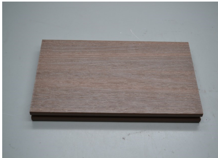
Fig 4. After salt spray test
